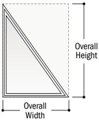
**Right triangles** contain one 90° corner. Specify overall width and overall height extending from the 90° corner.
