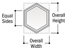
**Hexagons** contain six equal angles and sides. Specify length of equal sides.
