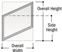
**Parallelograms** contain two pairs of parallel sides. Specify overall width along with side height and overall window height.
