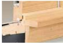
A clear pine stool is available and ready for finishing. The Woodwright stool is available in 4 9/16" (116) for use in wall depths up to 5 1/4" (133) and 6 9/16" (167) for use in wall depths up to 7 1/8" (181). Works with 2 1/4" (57) and 2 1/2" (64) casing widths. Shown above on a 400 Series tilt-wash double-hung window.
