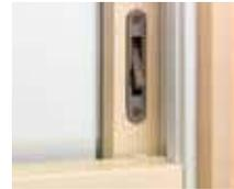
A recessed window opening control device is available factory applied. It limits the sash travel to less than 4" (102) when the window is first opened. Available in white, stone and black. A field-applied window opening control device kit is also available.
