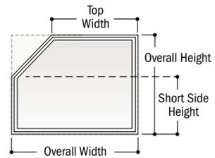
**Angled pentagons** contain an angle cut, or a "cut-off corner" sloping to left or right. Specify overall width and top width along with short side height and overall height.
