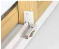
A window opening control device is available, which limits sash travel to less than 4" (102) when the window is first opened. Available in factory applied, or as a field-applied kit in stone or white. Device shown above on a 200 Series gliding window.
