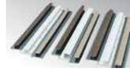
Rigid vinyl "J" and "h" channels are available in white, Sandtone and Terratone. "J" and "h" channels are 1/2" (13) deep and come in 150" (3810) lengths. "J" channels are 3/4" (19) wide and "h" channels are 1" (25) wide. "H" channels are 3/4" (19) deep and come in 84" (2134) and 150" (3810) lengths. White "H" channels are 3/4" (19) wide. Sandtone and Terratone "H" channels are 1" (25) wide.
