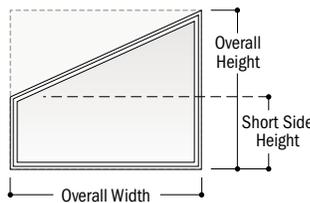
**Trapezoids** contain an angle face cut to left or right. Specify overall width along with short side height and overall height. Window's pitch is often designed to match a roof's pitch.
