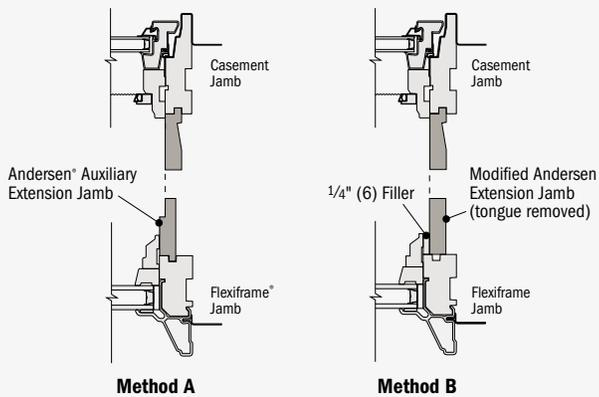
**Method A: Individually Framed** – Use optional Andersen auxiliary extension jambs for individual picture frame trimming.
