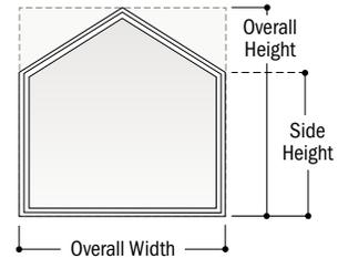
**Peak pentagons** contain sides of equal length extending at right angles from the sill and two angled sides of equal length that peak above center of sill. Specify overall width, side height and overall height.
