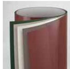
Andersen® aluminum coil stock can be ordered to match any of our 11 trim colors. Made from .018" thick aluminum, Andersen coil stock is available in 24" (610) x 50' (15240) rolls. Color-matched 1 1/4" (32)-long stainless steel trim nails are also available and can be ordered in 1 lb./454 kg boxes.
