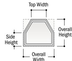
**Unequal hexagons** contain three pairs of angles and two sets of equal-length sides. Top side is parallel to and centered over the sill. Specify overall width, top width, short side height and overall height.
