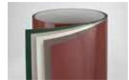
Factory finished in any of our 11 exterior trim colors, our aluminum coil stock allows you to form your own profiles in the field. Made from .018" thick aluminum, coil stock is available in 24" (610) x 50' (15240) rolls. Color-matched 1 1/4" (32)-long stainless steel trim nails are also available and can be ordered in 1 lb/.454 kg boxes.
