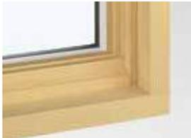
To help preserve original alignment of trim and paint lines in replacement situations, special 1 1/8" (29) thick replacement extension jambs are available. Factory-applied and non-applied extension jambs are available in 1/16" (1.5) increments between 4 9/16" (116) and 7 1/8" (181). Non-applied extension jambs are available in 12' (3658) lineals. Detail on page 34.
