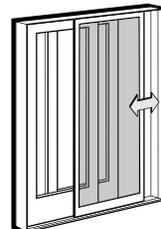
Patented square-corner joint construction adds considerable strength to the frame members. The insect screen is available for both two-panel doors and four-panel doors. Gliding insect screens have Delrin<sup>®</sup> injection-molded bottom rollers with self-contained leveling adjusters, providing smooth operation. Interior and exterior pulls and latch are provided.
