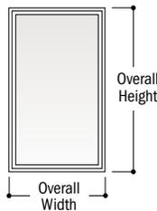
**Rectangles** contain four equal angles and two equal sides for rectangles, or four equal sides for squares. Specify overall width and overall height.
