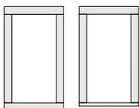
**Flat Casing** can be used on all four sides flush at the head and sill. Combine 3 1/2" (89) and 4 1/2" (114) flat casing or use with a flush sill nose.
