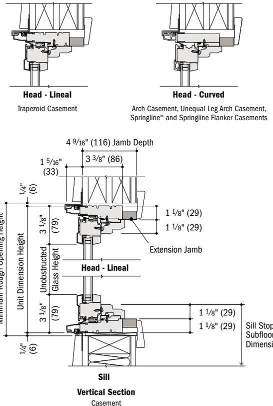
• 4 9/16" (116) overall jamb depth and 3 3/8" (86) base jamb depth measurement is from back side of installation flange.
