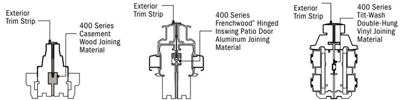
Reinforced joining materials are used to create product alignment, positive joining and load transfer between the Andersen windows and doors and the rough opening.
