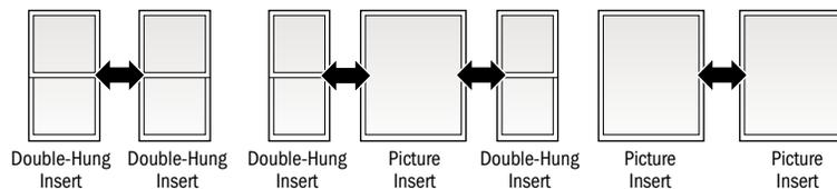
**Vertical (ribbon) Joining Detail**
