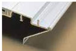
An aluminum sill support is designed to lock into a channel under the sill and tie back into the wall. This offers support to the outermost sill section when needed. Available in a neutral gray finish.
