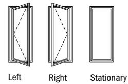
Choose left, right or stationary as viewed from the exterior. In addition to venting shown in table, other standard configurations are available for single, twin and triple windows. Transom (CTR) windows are stationary only.
