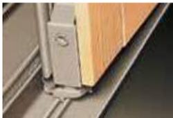
Teflon®-infused Delrin glides are self-lubricating and require only 8 lbs/3.6 kg of force to operate. A stainless steel spring within the glide provides years\* of reliable operation – even in harsh environments.
