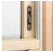
A recessed window opening control device is available factory applied. It limits the sash travel to less than 4" (102) when the window is first opened. Available in white, stone and black. A field-applied window opening control device kit is also available.
