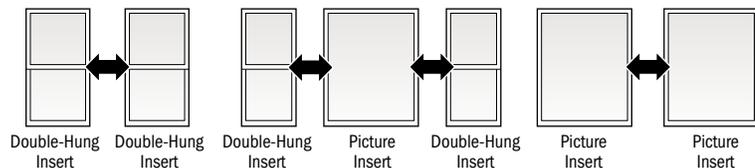
**Vertical (ribbon) Joining Detail**
