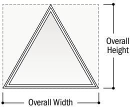
**Isosceles triangles** contain two sides of equal length and equal angle. Specify overall width and overall height (sill to peak).
