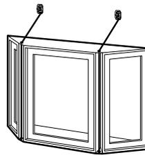
A cable provides additional support. Recommended for installations that extend out from the structure without a framed support wall beneath the unit. Each cable within the system can support a maximum load of 500 lbs/227 kg. If the section of the window unit requiring support exceeds 1000 lbs/554 kg, additional support is necessary. Failure to use sufficient structural support could result in personal injury or damage to windows or other property.
