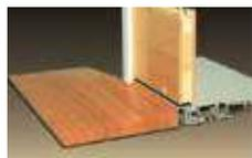
Ramped sills in maple or oak provide smooth transition from interior to exterior. Ramped sill cannot be used with insect screens. Check with local and federal officials to determine if product meets accessibility codes. Shown with a Frenchwood<sup>®</sup> gliding patio door.
