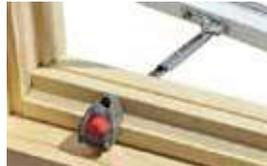
A window opening control device is available, which limits sash travel to less than 4" (102) when the window is first opened. Available factory applied, or as a field-applied kit in stone, white and black. Not available for French casement windows.
