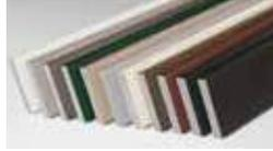
Available in the same 11 colors as our exterior trim, this solid cellular Fibrex trim board can be cut or ripped to size, and be fastened using nails or screws. 3 1/2" (89) x 3/4" (19) thick in 10' (3048) lengths.
