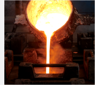
casting the escutcheon plate
