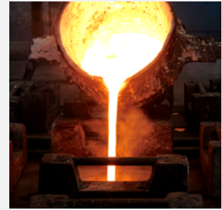
casting the escutcheon plate
