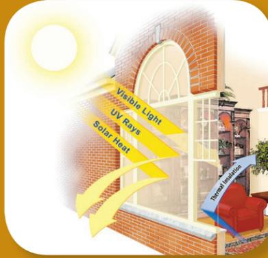
Low-E glass has a secondary, very thin metallic dual layer coating. This allows the sun's heat and light to pass through the insulating glass, but, at the same time, actually works to reflect radiant heat back toward its source. Since Low-E coating reflects radiant heat waves, it helps keep your home warmer in the winter by trapping radiant heat and cooler in the summer by blocking it from your home.
