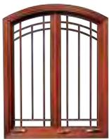
Andersen® complementary French casements allow both sash to swing outward from the center, eliminating a center mullion post. They offer smooth operating multi-point locking mechanisms and hinges. The multi-point lock is activated with a single turn of a handle that simultaneously secures both sash. French casement windows have a unique locking handle that's available in antique brass, black, bright brass, oil rubbed bronze, satin nickel, stone and white finishes.
