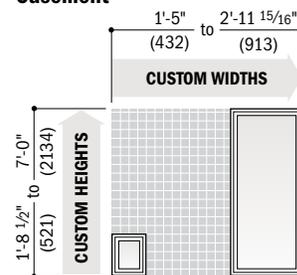
\* Rough openings may need to be increased to allow for use of building wraps, flashing, sill panning, brackets, fasteners or other items. See pages 226-227 for more details.
