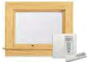
Awning windows can be ordered with an operator enhanced by PowerAssist™ technology that opens and closes the window with the touch of a button. Easy to install, the 24-volt system features a concealed window power driver, battery backup in case of a power outage, and a moisture sensor that automatically closes the window when it rains. A wireless remote control is available (sold separately).
