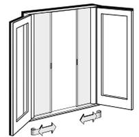
**Retractable insect screen** for two-panel outswing doors. Installed on the interior, it neatly retracts into a small canister.
