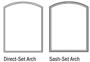
**Direct-set arch (ATAD) window sizes shown.** Use window dimensions and minimum rough opening formula shown for sash-set arch (ATA) window sizes. For sash-set unobstructed glass dimensions, see pages 94-97. All sizes shown, along with custom sizes, are available with PG upgrade.
