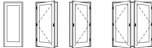
**Stationary** (non-operating panel)    **Left Hinged** (hinges on left)    **Right Hinged** (hinges on right)    **Active Panel** (operating panel used most often)    **Passive Panel** (operating panel with attached astragal)
