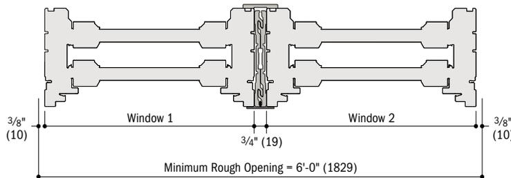
For factory-joined windows, modular sizing allows for easy calculation of minimum rough opening sizes.
