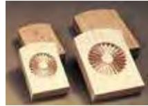
For arch windows with 2 1/4" (57) and 2 1/2" (64) casing, use 2 7/8" (73) x 4" (102) size plinth block. For arch windows with 3 1/2" (89) casing, use 3 7/8" (98) x 5 1/4" (133) size plinth block.
