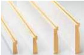
Extension jambs are available in pine, maple, vertical grain Douglas fir, oak, mahogany\* and cherry, precut to fit the unit. Available in 1/4" (1.5) increments up to 7 1/8" (181) and can be prefinished in six stain colors as well as all interior paint options to match the interior of the unit. This option is also available factory applied.
