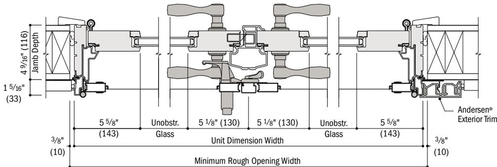
**Horizontal Section – Two-Panel Active-Passive (APLR/PALR)**
