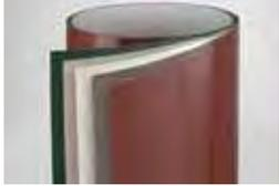
Andersen aluminum coil stock can be ordered to match any of our 11 exterior trim colors. Made from .018" thick aluminum, coil stock is available in 24" (610) x 50' (15240) rolls. Color-matched 1 1/4" (32)-long stainless steel trim nails are also available and can be ordered in 1 lb/454 kg boxes.
