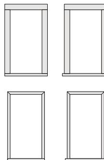
**Sill Nose** can be used with flat casing or brick mould. It can be applied flush or extended.
