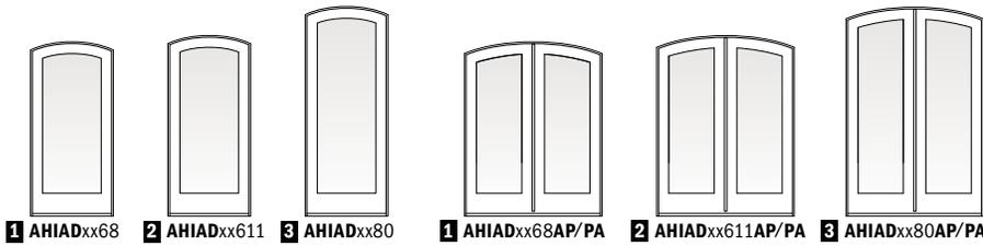
Custom-size doors are available in 1/8" (3) increments. Traditional panels are standard. Custom-designed and 3/4-light panels are also available. Stationary doors are also available (i.e., 2168S or 4068SS). Add AHIAH to "Door Number" listed in table (i.e., AHIAH2168).
