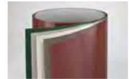
Andersen aluminum coil stock allows you to form your own profiles in the field and can be ordered to match any of our 11 exterior trim colors. Made from .018" thick aluminum, coil stock is available in 24" (610) x 50' (15240) rolls. Color-matched 1/4" (32)-long stainless steel trim nails are also available and can be ordered in 1 lb/454 kg boxes.
