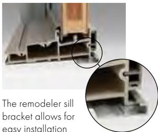
The remodeler sill bracket allows for easy installation in replacement applications with a finished interior floor. It fastens to the subfloor, and the sill snaps into the bracket, providing a secure structural installation. Detail is shown on page 129 for gliding, 141 for inswing and 153 for outswing doors.
