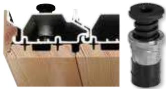
Built-in jacking screws make installation easier. Jacking screws positioned within side and head jambs serve as built-in shims enabling fine adjustments during installation. Precision adjustments enable frame and panels to interact as designed during initial installation and throughout the life of the product for smooth operation.
