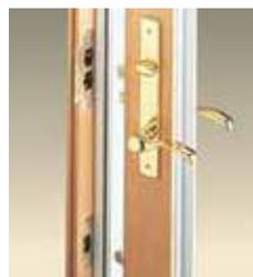
The folding outswing door has a multi-point locking system with a hook bolt above and below the center deadbolt along with flush bolts on the panels that lock into the head and sill. This system provides a weathertight seal and enhanced security. The flush bolts and pull handles are available in a matte black or satin stainless steel finish.
